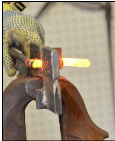
Tong jig in use.
