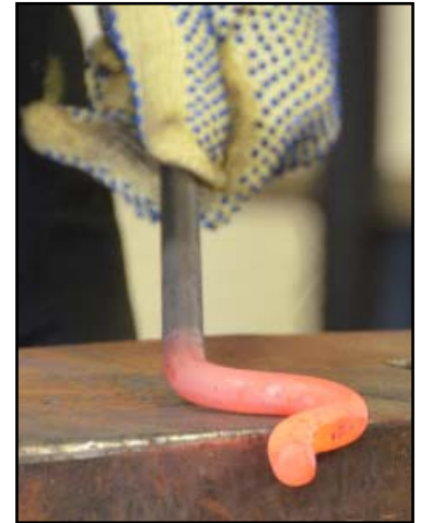
Round bar formed by jig.
