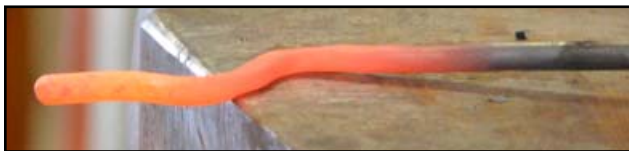
Tong half, boss has been flattened and jaws being worked. Shown at a different angle below.
