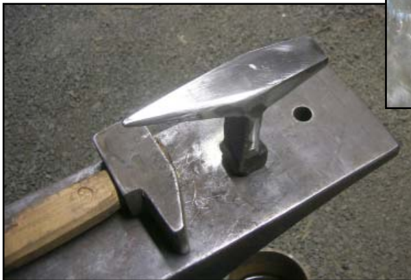
7. The stake anvil installed on top of 200# TFS anvil.
