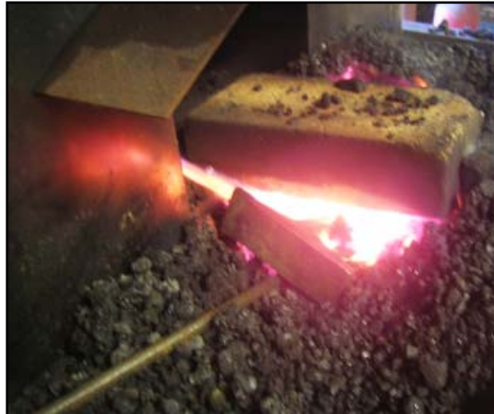
2. Slice of RR rail in the fire with \frac{3}{8} rod welded to it for handling without tongs. The fire brick is to hold in the heat like a little oven.
