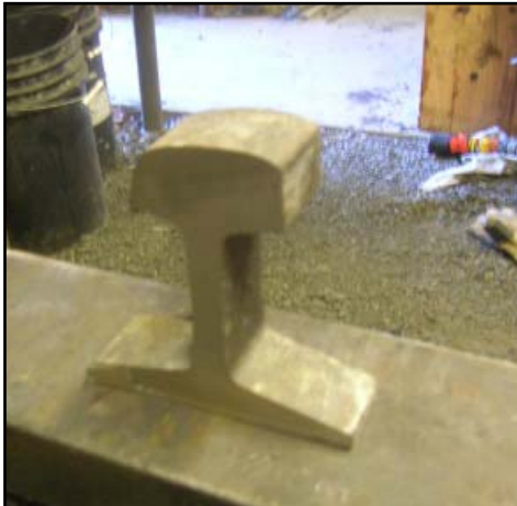
1. Slice of RR rail to make a stake anvil. I cut this off from the rail shown in the last photo.
