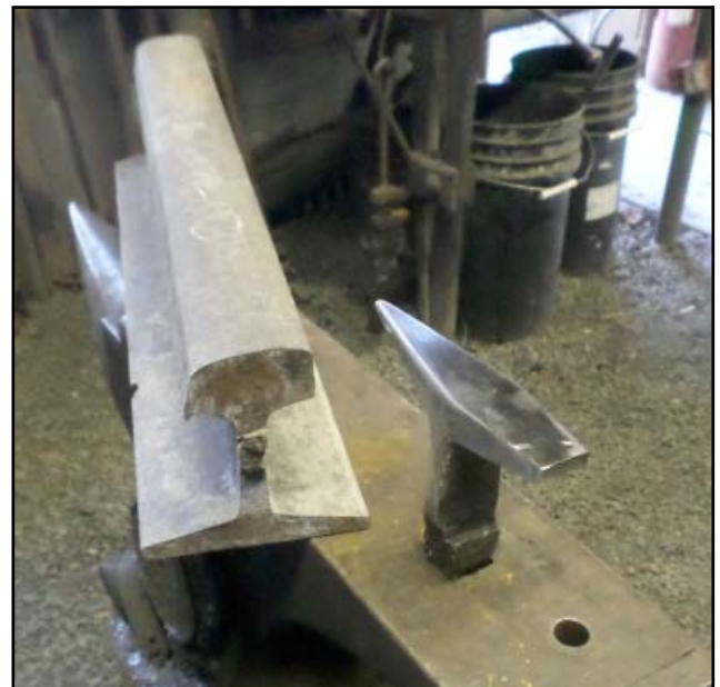
This stake anvil was made from a slice of this RR rail.
