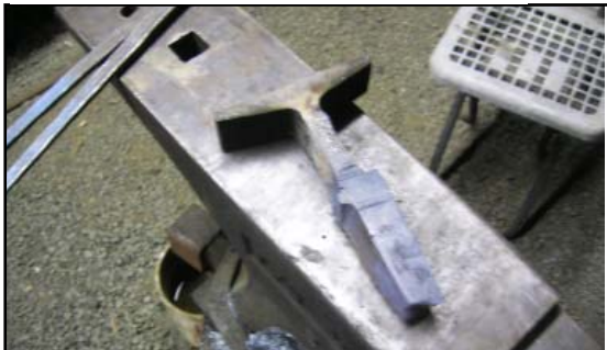
4. The hardy is drawn out, ready to start fitting in the hardy hole.
