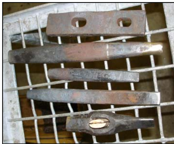
Bottom to top: handled punch, hand-held punch, large and small drifts and bolster
