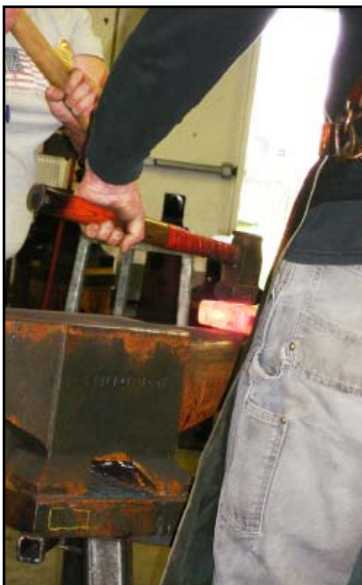
Using the fuller to form the pien.
