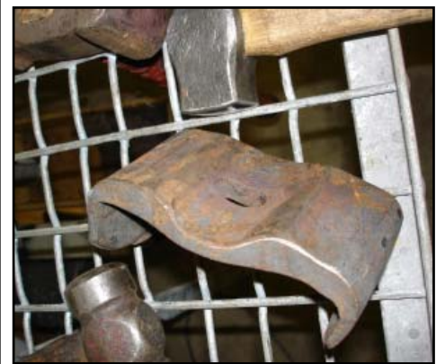
Curved bolster as an anvil saddle
