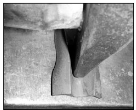
Step 6: Flip channel and fuller back approximately 2 1/2"
