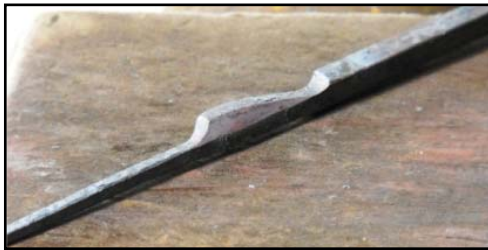
5. Hold the second section diagonally and flatten to 3/16".
