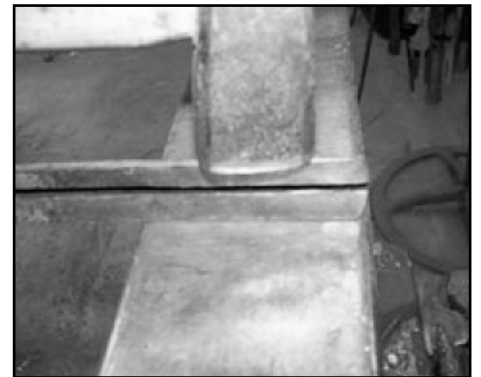
Step 3: Further narrow opening by edge hammering
