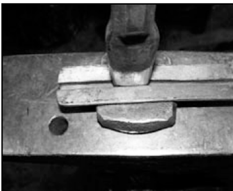
Step 4: Redefine opening using 1/4" flat bottom chisel in hardy
