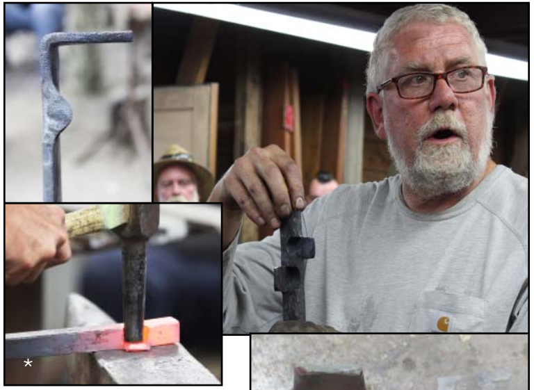
Above and Right: Pulling a tab out by cutting with a 1/2 round gauging chisel, setting with flat faced top tool, keeping the edge of the tab heavy at first. Many uses and styles were shown, flat bar and square stock. Joe shows how angling the tabs in opposite direction on square stock can be used as an integrated solution for table leg fastening.
