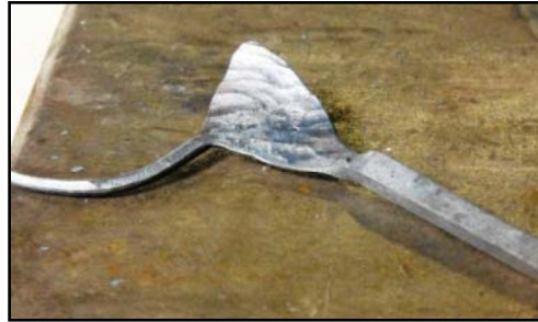
8. Concentrate on spreading body perpendicular to stock.
