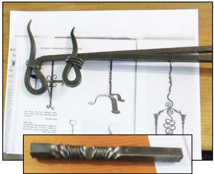
Martin Brandt, left facing forward, demonstrated lots of twist techniques, from the simplest to quite fancy. Practicing twists is a great way to learn about how hot steel moves, it doesn't always turn out as expected, but the results are informative
