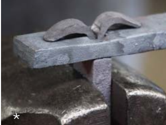
Left and above: Decorative tenon fastening. Draw out the tenon, split it in two, pass it through the pierced bar, and pry it open to snug up the joint, and scroll ends decoratively.
