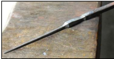
4. Draw first section to 4 1/2"+, round if desired.
