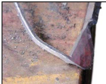
7. Using either the radius edge of anvil or hammer peen, begin to spread body of shell.
