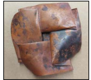
After radial lines are broken to ~ 45Degrees the 'Vessel' is inverted on flat plate and compressed with set hammer placed on flat of the central square. You can compress to flat or leave as a 'Vessel' form. The final closing may be coaxed by hand, correcting with hammer as needed.
