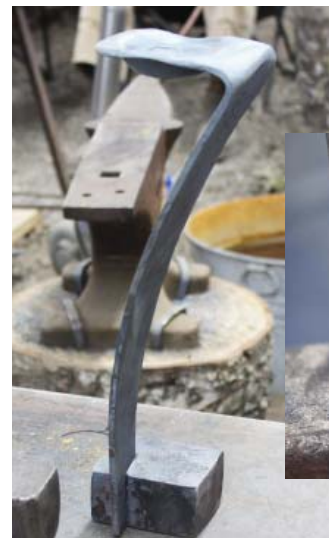
Above: Stylized candlestick. Tapered flat stock bowled on a swage at the wide end, creating the candle cup. Heavy base cut to a depth of approximately 2/3 the width of the flat stock. Pierce the flat stock where it fits the base, 2 perpendicular holes will help lock the joint when the cold flat bar is slid into place in the hot base and the base is hammered closed. This is the joint named The Joe Joint.
