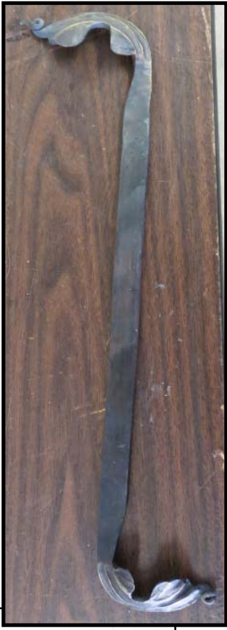
Lisa's sample Italian Leaf in steel, left end is complete, right end a leaf in progress.
