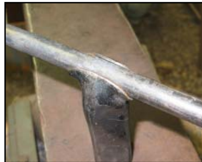
Left and above: Decorative tenon fastening. Draw out the tenon, split it in two, pass it through the pierced bar, and pry it open to snug up the joint, and scroll ends decoratively.
