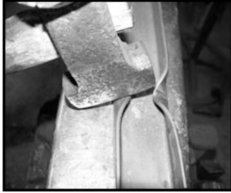
Step 2: Fuller in at the 2 1/2" mark
