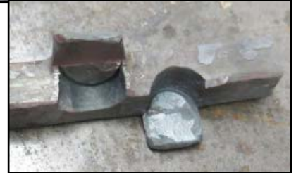
Above and Right: Pulling a tab out by cutting with a 1/2 round gauging chisel, setting with flat faced top tool, keeping the edge of the tab heavy at first. Many uses and styles were shown, flat bar and square stock. Joe shows how angling the tabs in opposite direction on square stock can be used as an integrated solution for table leg fastening.
