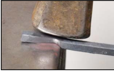
1. Using 3/8" sq. place 1" on face holding the steel at a slight angle to anvil face and apply half face hammer blows on two sides reducing to 3/16" at anvil edge.
