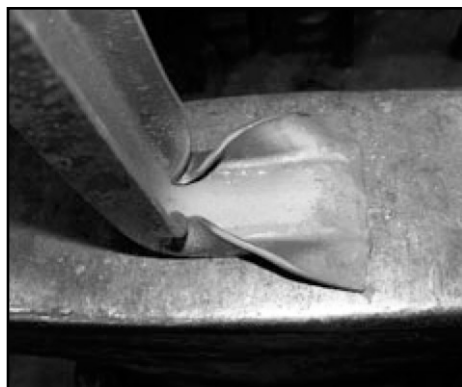
Step 5: Bend foot over anvil edge and true to 90 degrees
