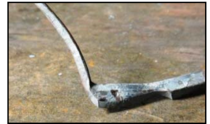
6. Clamp flattened section in vice and bend tang away from mass to 90°.
