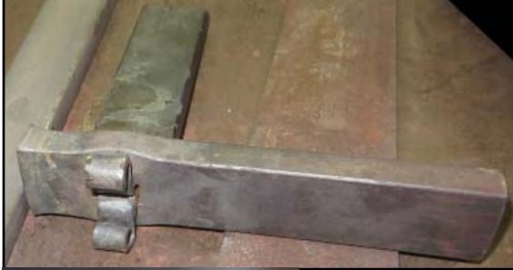
Left and above: Decorative tenon fastening. Draw out the tenon, split it in two, pass it through the pierced bar, and pry it open to snug up the joint, and scroll ends decoratively.
