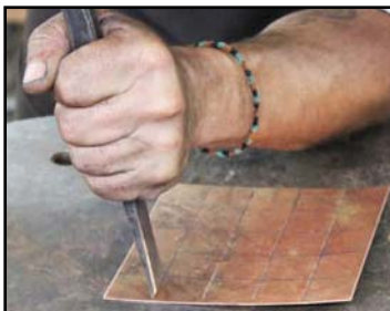
Design transferred to one side, use cold chisel on valley side only. Cut up to but not onto the intersections of the valley lines, and keep away from all edges
