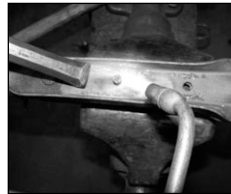
Step 8: drill holes and set 5/16" rivets to secure body portion
