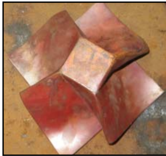
Work vessel sides to 90° with hammer, form past that by hand. As before, take care to keep lines crisp, frequent annealing, work evenly all around.
