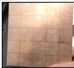
Drawing on the left above is the repeated tessellation and as folded (dotted lines fold to valleys, solid lines to peaks), as transferred to copper sheet, and tessellation fit to 5 x 5 grid, X's are the valley lines. Use lighter material, 20 gauge, when making a complex pattern with many folds.
