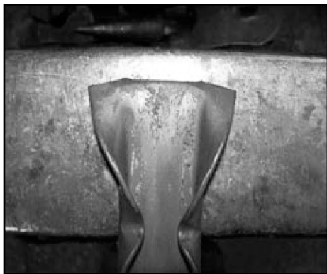
Step 4: Further spread webs over anvil face
