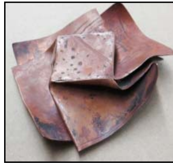
After radial lines are broken to ~ 45Degrees the 'Vessel' is inverted on flat plate and compressed with set hammer placed on flat of the central square. You can compress to flat or leave as a 'Vessel' form. The final closing may be coaxed by hand, correcting with hammer as needed.
