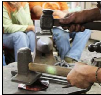
After radial lines are broken to ~ 45Degrees the 'Vessel' is inverted on flat plate and compressed with set hammer placed on flat of the central square. You can compress to flat or leave as a 'Vessel' form. The final closing may be coaxed by hand, correcting with hammer as needed.
