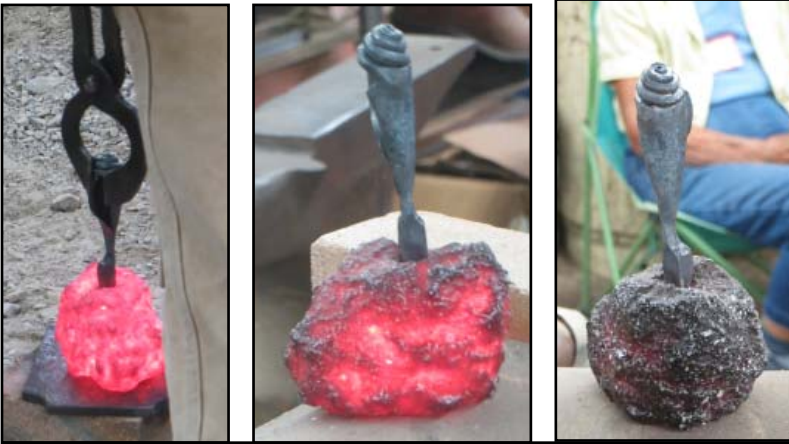
Forgable rocks preheating atop the forge.
