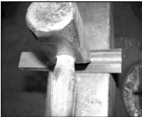
Step 1: Open channel with cross peen over anvil face
