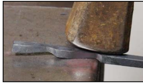
2. Advance steel onto anvil face another 1" and repeat process.
