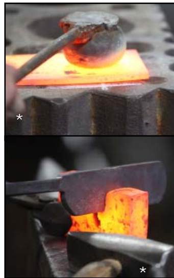
Above: Stylized candlestick. Tapered flat stock bowled on a swage at the wide end, creating the candle cup. Heavy base cut to a depth of approximately 2/3 the width of the flat stock. Pierce the flat stock where it fits the base, 2 perpendicular holes will help lock the joint when the cold flat bar is slid into place in the hot base and the base is hammered closed. This is the joint named The Joe Joint.
