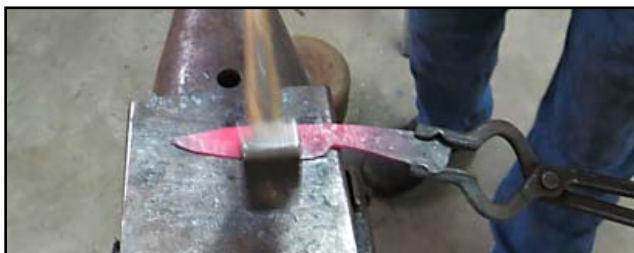
Beveling and tapering the blade.
