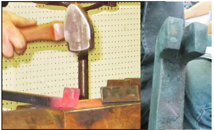
Above and Below: Creating the square corner for the lock body, cutting the tabs and fullering the bottom of the cut.
