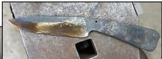
Above: Nice colors of the tempered blade.
