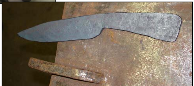
Photo right by Hardy Swage: the roughed in blade
