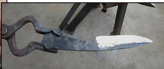
Dressing profile and bevel with grinding tools.
