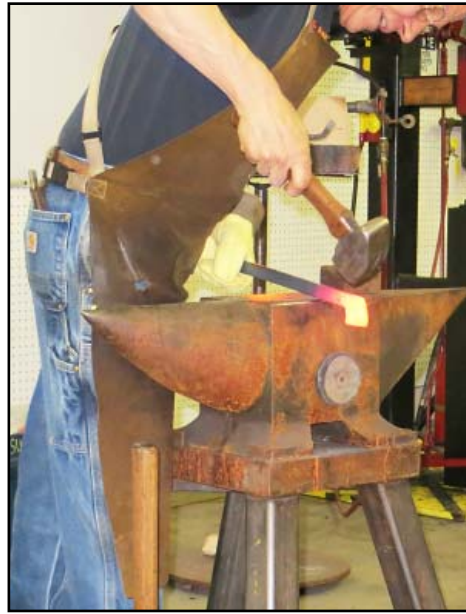
Above and Below: Creating the square corner for the lock body, cutting the tabs and fullering the bottom of the cut.
