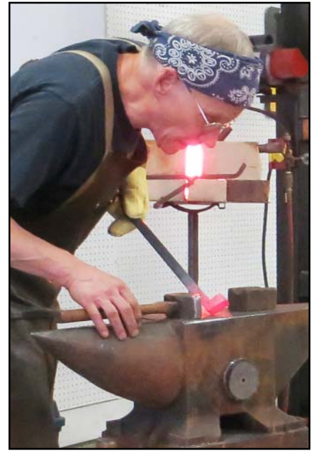
Above and Below: Creating the square corner for the lock body, cutting the tabs and fullering the bottom of the cut.
