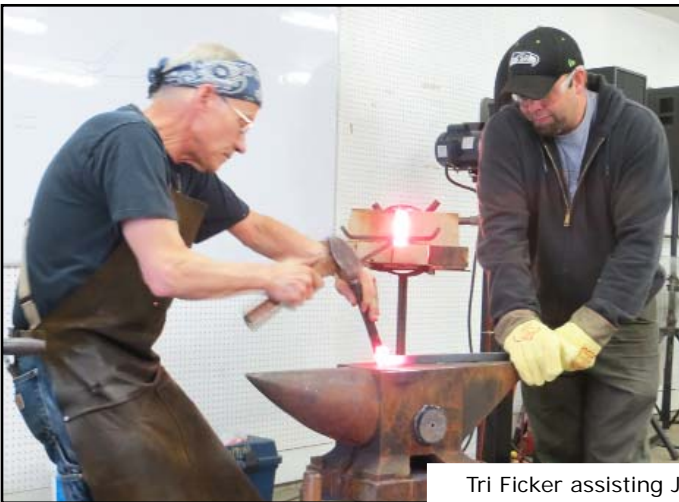
Above and Below: Creating the square corner for the lock body, cutting the tabs and fullering the bottom of the cut.
