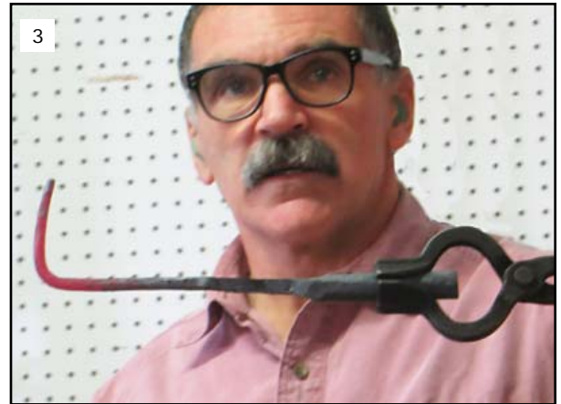
3. First of 2 bends, gently begin the second bend approximately halfway between the first bend and the punched and drifted hole, working the tip of the taper into the hole.
