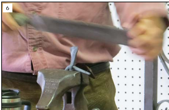
6. Rasp it smooth. This happened so quickly and deftly that there were no photos of the steps between cutting and rasping.
