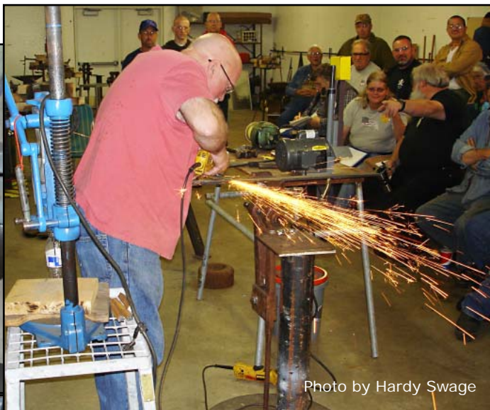
Dressing profile and bevel with grinding tools.
