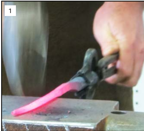
1. Lay off 5" of bar, work it down lightly, giving it a little flavor. Round it up after going octagonal (8 equal sides). Aim for 6 1/4" in length forged stock (6 1/2" is ok).
