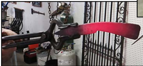
Photos above: Beginning rough forging steps.
