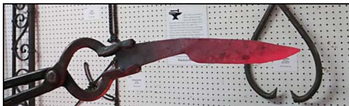
Beveling and tapering the blade.
