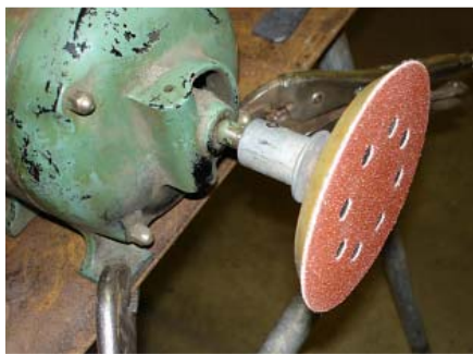
Hook & Loop 5" soft pad and abrasive discs on a 1750 RPM motor.
