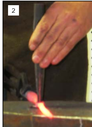
2. Punch a hole in fatter end of the taper, and drift to ~3/8"
