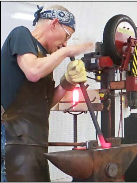
Above and Below: Creating the square corner for the lock body, cutting the tabs and fullering the bottom of the cut.
