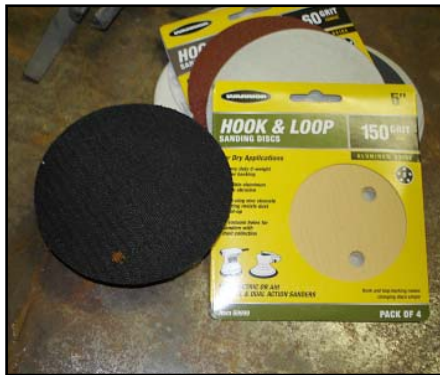
Hook & Loop 5" soft pad and abrasive discs on a 1750 RPM motor.
