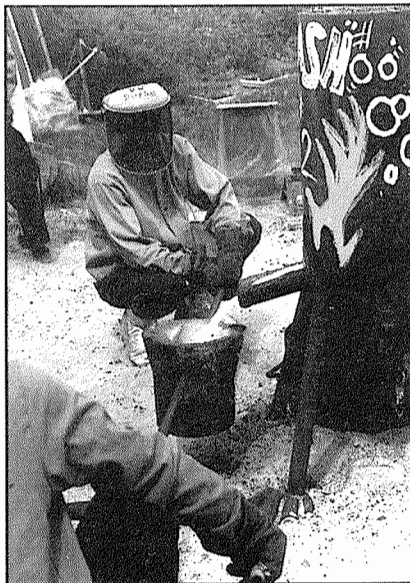
"Tapping out", filling the ladle with hot iron.
