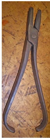
Right: Scrolling tongs with box joint – more robust than pliers
