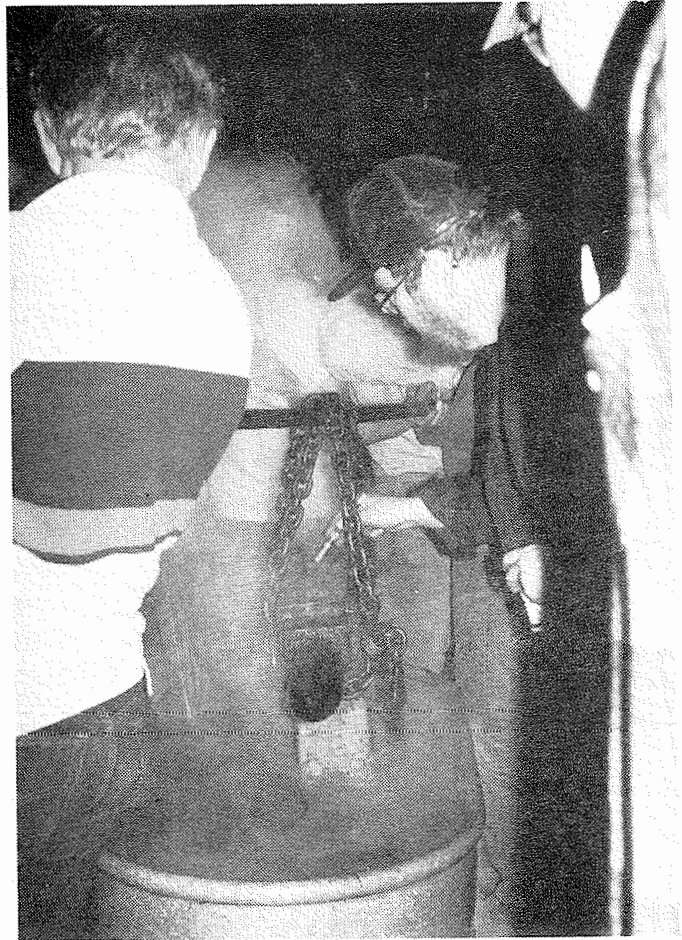
Gene Chapman applies tempil stick to anvil to ascertain heat, as anvil is lifted from tank.
