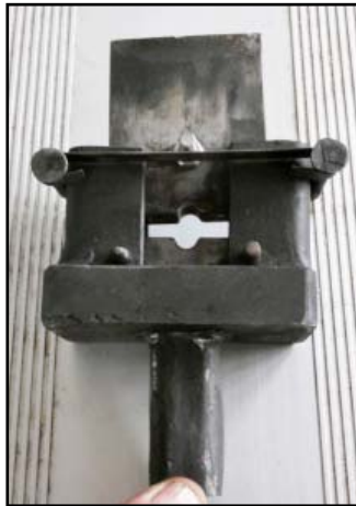
Swaging the shoulder rivet pin with a guillotine swage.
