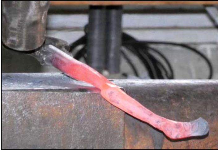
Forging legs, comparing often to make a matching pair.
