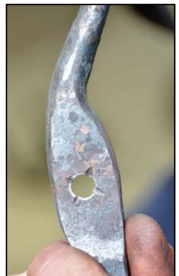
Boss/handle transition well started.
