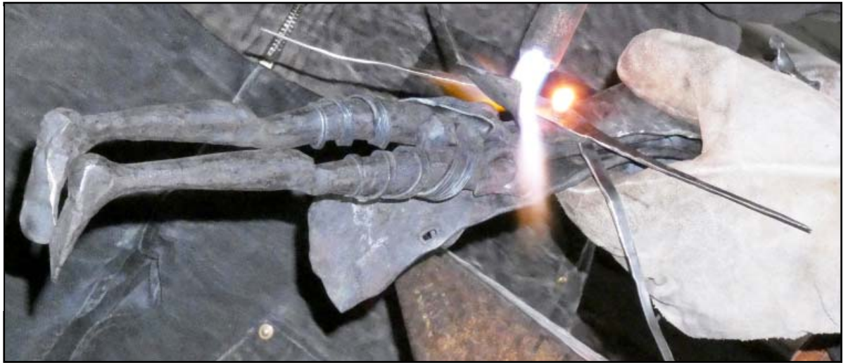
Arms get divots for rivets, and are attached at the shoulder rivet pins.
