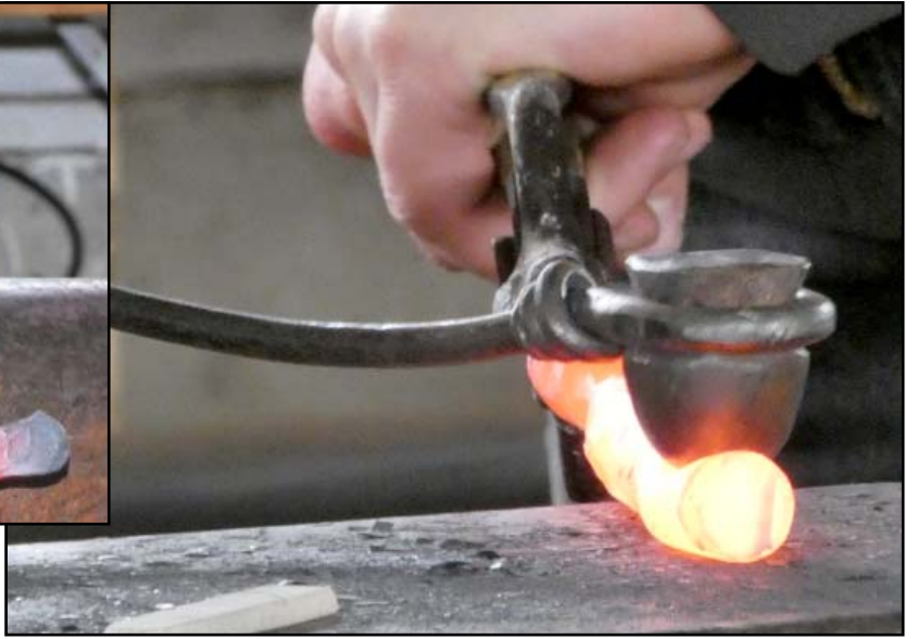
Creating the inset where the rivet will go when attaching the leg to the body core.
