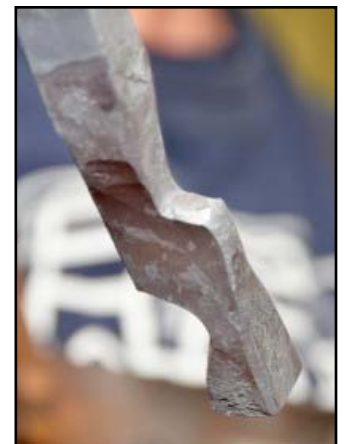
Boss/handle transition well started.
