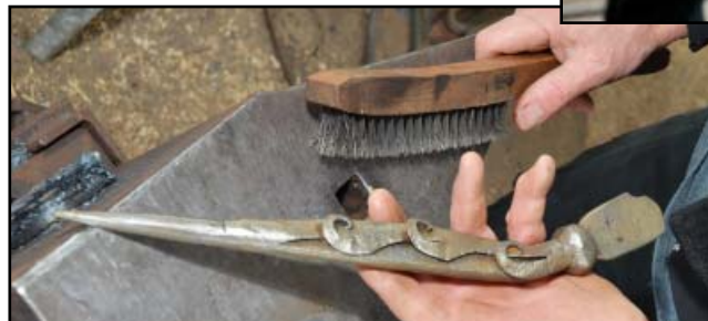
Used last of welding heat to cant back end. Note pickle finish, piece soaked overnight in phosphoric acid solution.
