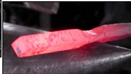
Fullering bottom (fat) end of body core and cutting it to length.
