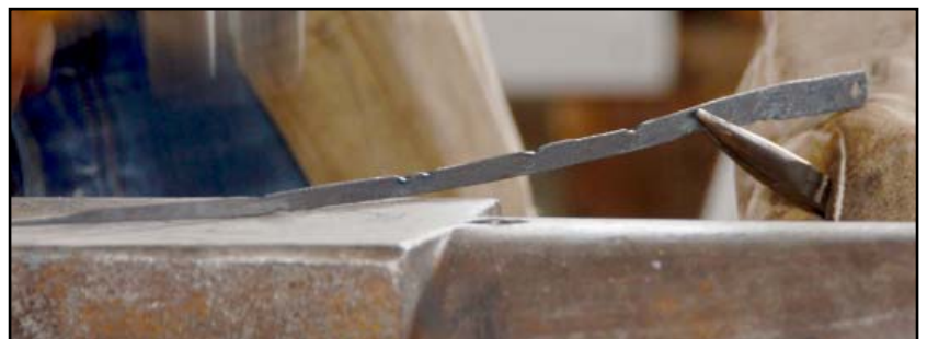
Left: Texturing swage used to texture winding straps. The straps will be used to wrap body and wrap around legs.
