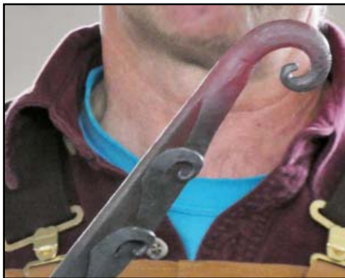
Forging centered tang, ~1/4" thick.
