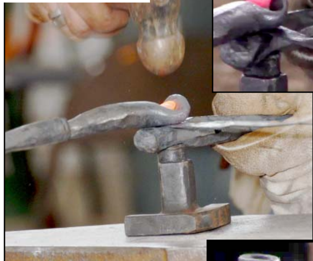
Riveting leg to body core, textured wrapping strap in between body core and leg, not easily visible in these photos.
