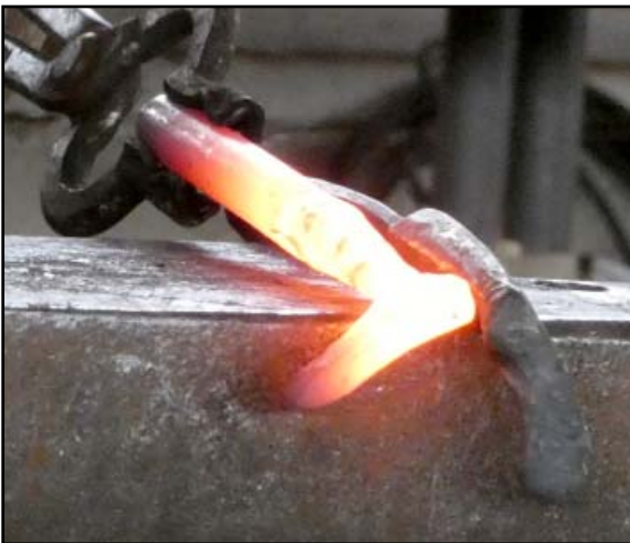
Forging legs, comparing often to make a matching pair.
