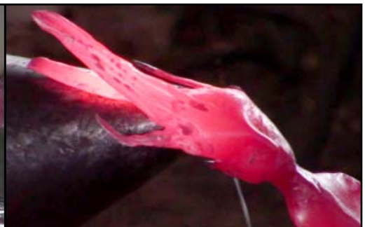
Forging the facial features. Tubing bolted to stock as a means of holding it in the vise.
