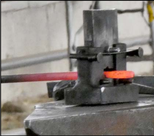
Swaging the shoulder rivet pin with a guillotine swage.
