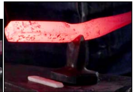
Fullering bottom (fat) end of body core and cutting it to length.
