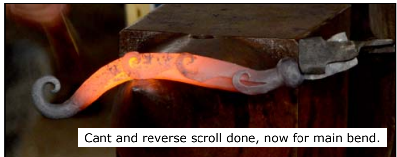
Used last of welding heat to cant back end. Note pickle finish, piece soaked overnight in phosphoric acid solution.
