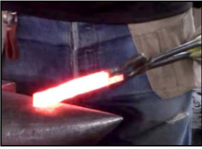
Forging body core.
