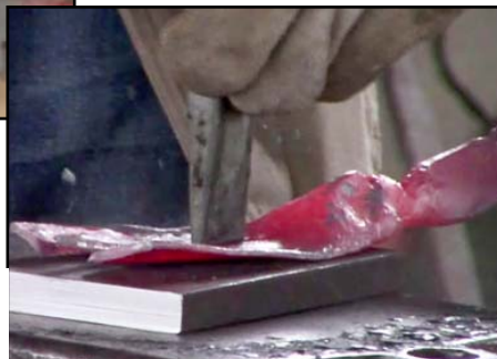
Forging the facial features. Tubing bolted to stock as a means of holding it in the vise.
