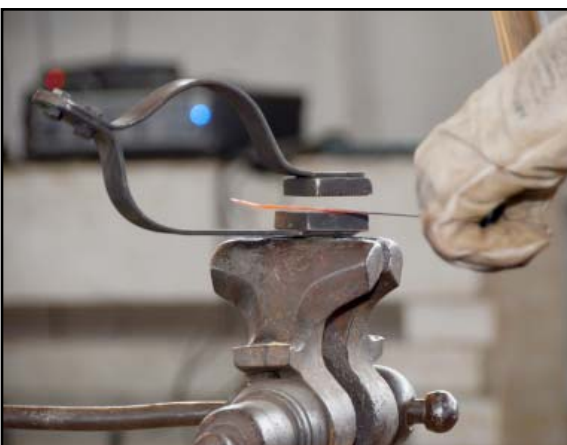
Left: Texturing swage used to texture winding straps. The straps will be used to wrap body and wrap around legs.
