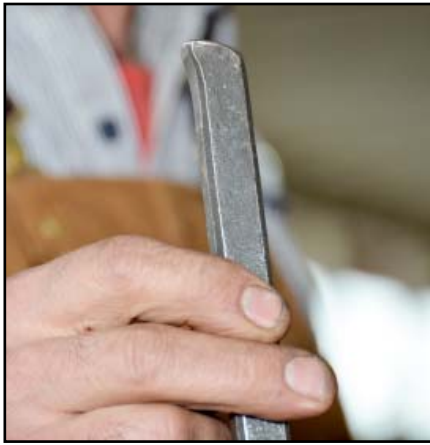
"Deer hoof" tool used for bending ears, pushes without marring.
