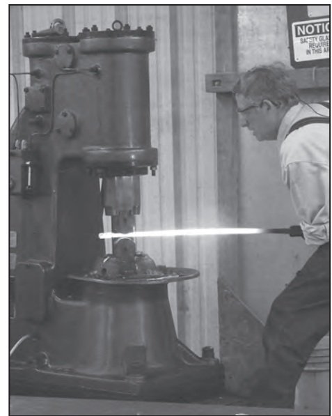
Berkley Tack on the Stryker 88. "Take little bites." "If you see your die even slightly out of line stop before it pops out."
