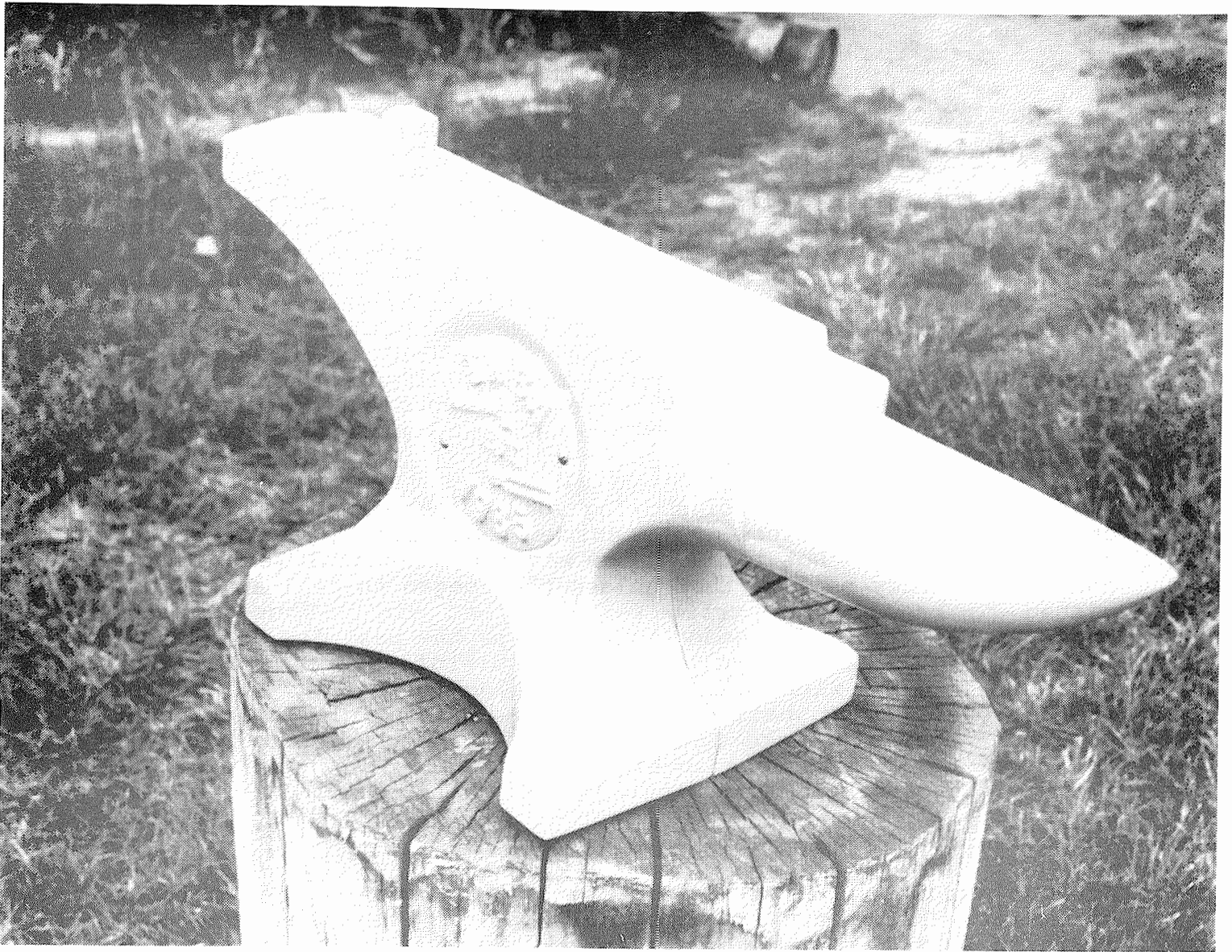
Above: FORM TO BE USED IN CASTING THE INBA ANVILS photo by Clayton Carr
