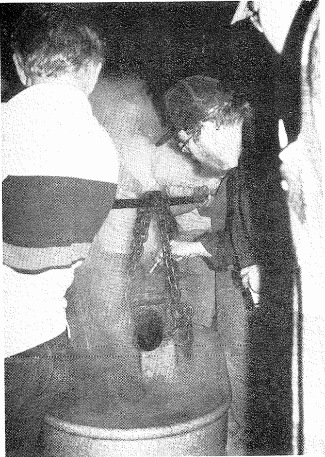
Gene Chapman applies tempil stick to anvil to ascertain heat, as anvil is lifted from tank.
