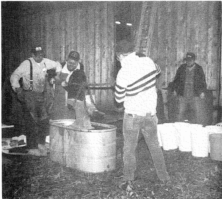
Gene Chapman applies tempil stick to anvil to ascertain heat, as anvil is lifted from tank.
