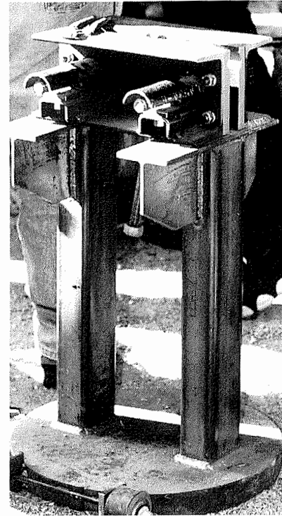
Dick Naven brought his twin screw chain driven vise for us to admire. Note the wheels on the base for ease in moving. This vise was used at the main demo site.
