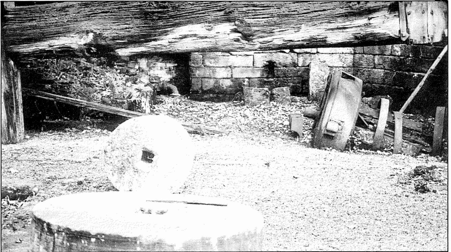
The East Hammer at the Mousehole Forge. The large log, circa 1780, supported the wooden spring that gave the tilt or helve hammer more power. The Five-Cam Wheel that lifted the Helve Hammer can be seen. The grinding stones were used to grind the anvil faces. The wheel pit for the stones is to the left of the stones. The forge for the helve hammer was on the other side of the log to the left at the back of the building.
