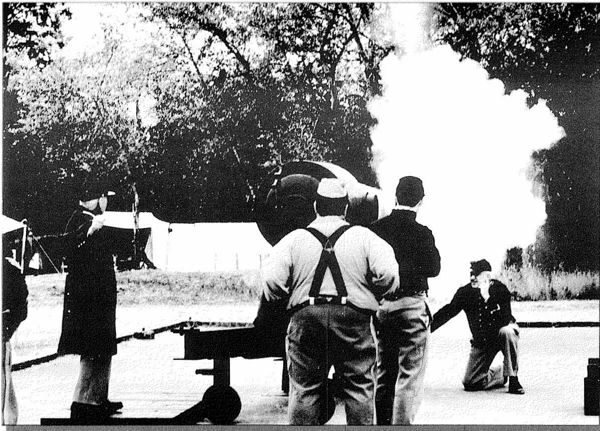
An 8-inch Parrott Rifle cannon barrel weighs 16,300 pounds and can fire a 175-pound shell over 8000 yards.
