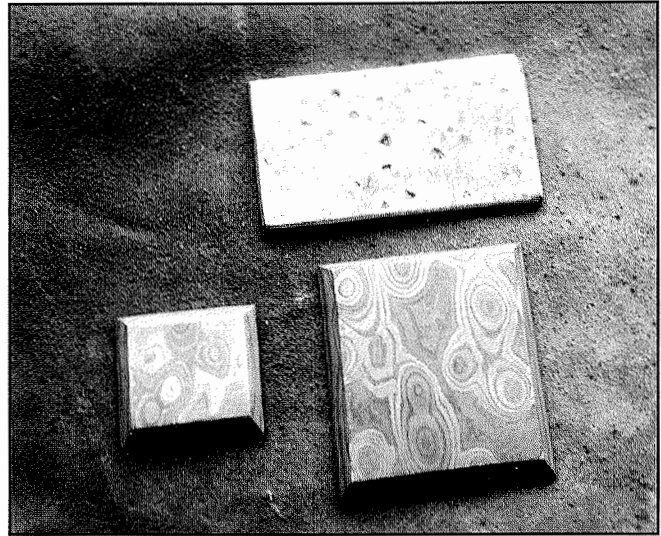
Top: Brass/Copper billet Bottom: Wrought iron
