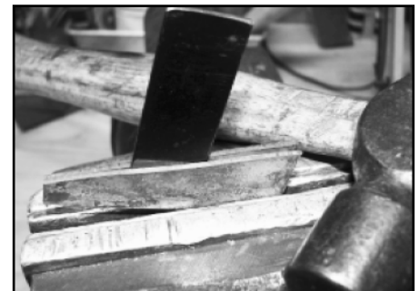
Gently open the handle with the skinny wedge.
