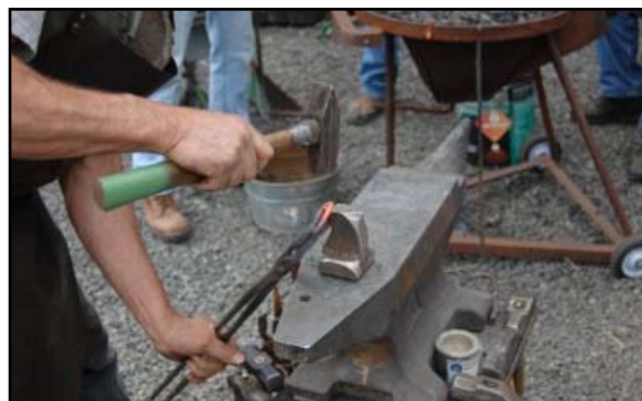
Forge welding a chain link
