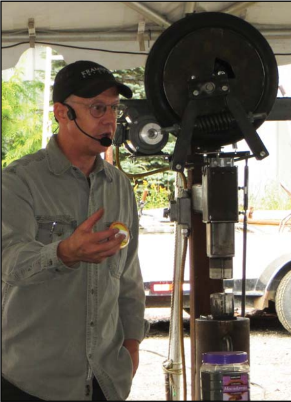
Bob Kramer demonstrating at Western States Blacksmith Conference 2013. Featured on the cover and above is a tire power hammer made by Larry Langdon. At the October 26, 2013 Board meeting it was voted to purchase a similar power hammer from Larry to have as part of our Mentoring Center equipment and to use at future conferences.
