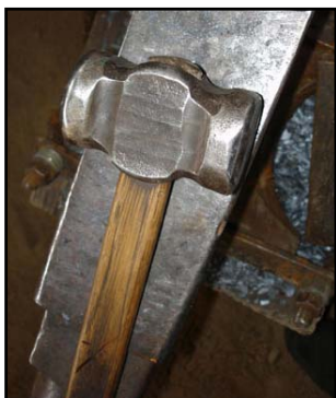
A forging hammer from round stock (wrist pins from truck repair shops make good inexpensive material source)
