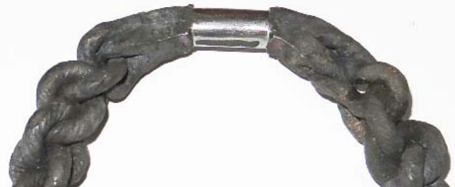
Forged welded section ground and polished to assure a smooth working hinge.
