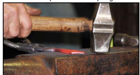
The thickness of the handle should be kept flat but can have a taper toward the top edge.
