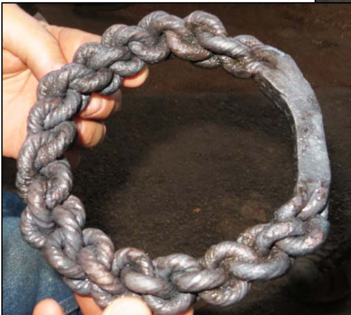
'Braided' Pull, made of all simple twists, gives the appearance of braided rope.
