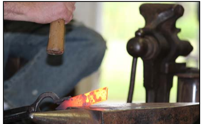
Use angle hammer blows to contour underside of the handle for a more comfortable feel for the fingers.
