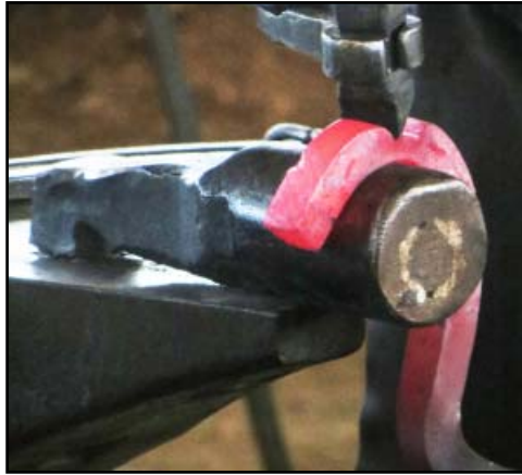
Flatten the base of the mortise. The flatter is smaller than the finished notch floor, move around to get the totally flat floor desired, angling the flatter to follow the layout and cuts.
