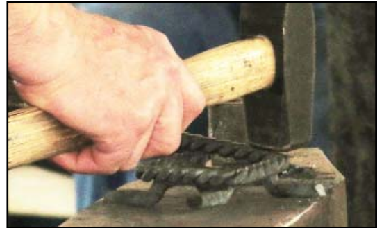
Trim piece made by twisting two 1/4" rods twisted together and forged square down to 3/8" sq., ends tig welded where collar would cover. Tap trim down into place.
