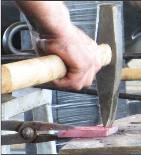
3" flat bar x 3/8". Strike a line ~3/8" from the edge.
