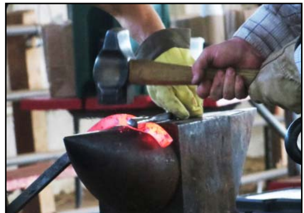
Flatten the bend at a high heat and with tenon form tool in place. Tenon pattern tools are made in swage for uniformity and consistency. This tool has an end profile of a dovetail but tapered.
