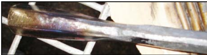
Flatten the bend at a high heat and with tenon form tool in place. Tenon pattern tools are made in swage for uniformity and consistency. This tool has an end profile of a dovetail but tapered.
