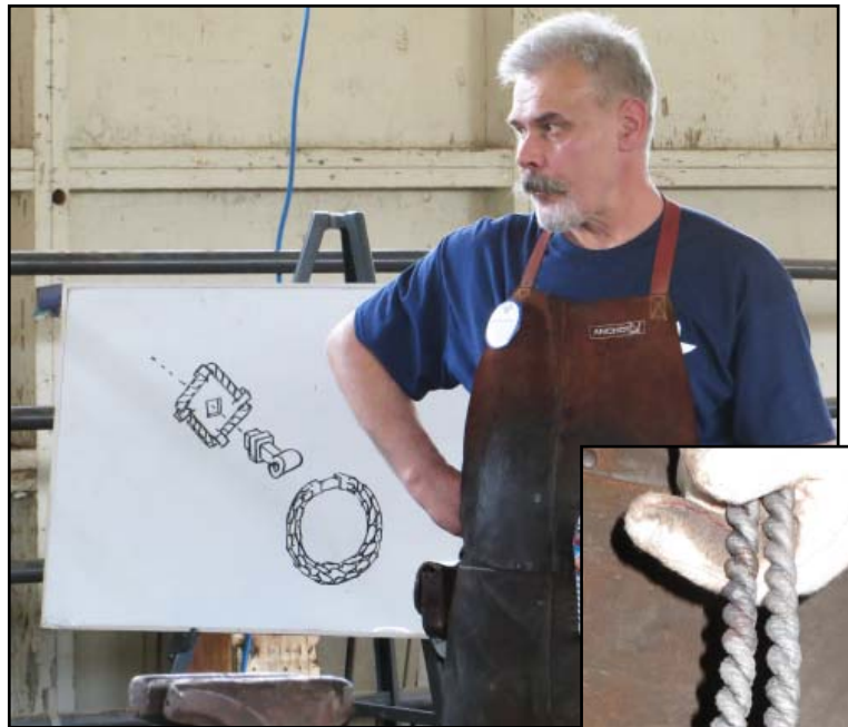
Beginning with the ring: 3/8" sq. stock, mild steel, ~3 1/2 - 4ft. Two pieces - same procedure. Round the pieces except for the ends and the center, bend in half, and hammer flat at the fold.
