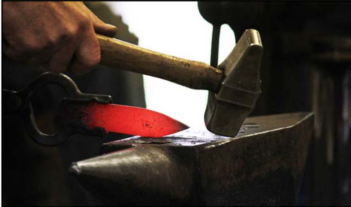
Using a well rounded edge of the anvil hammer a nick into the edge of the blank at the marked location.
