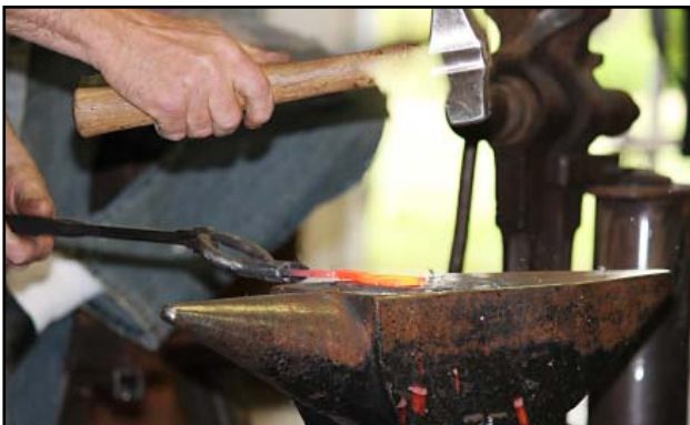
The horn of the anvil can also be used for this contouring.
