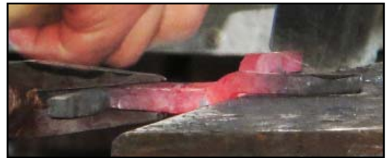
Offset the collar legs so the trim can sit flush with the plate.
