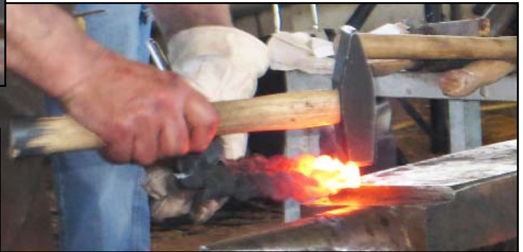
Use bending forks in vise and heat and curve over anvil horn using mallet to form the ring. Forge weld ends together.
