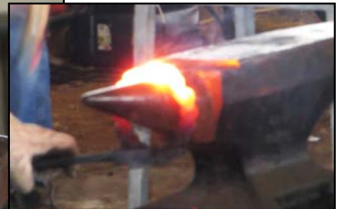
Use bending forks in vise and heat and curve over anvil horn using mallet to form the ring. Forge weld ends together.
