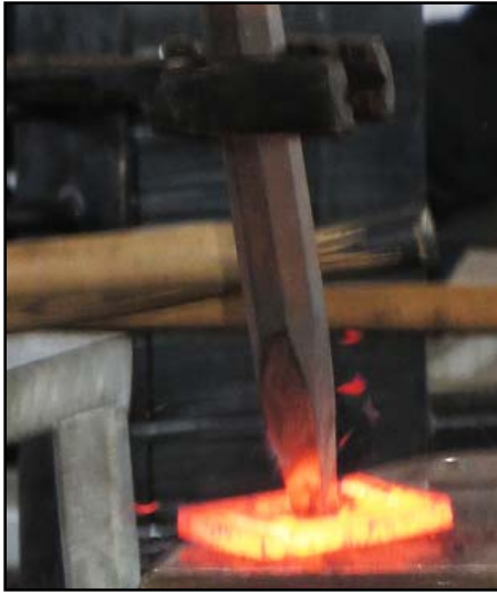
Cut a square hole on the diagonal, drift hole to make it larger.
