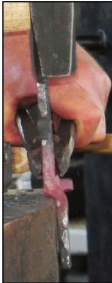
Trim piece made by twisting two 1/4" rods twisted together and forged square down to 3/8" sq., ends tig welded where collar would cover. Tap trim down into place.
