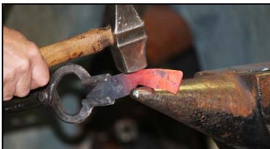
The horn of the anvil can also be used for this contouring.
