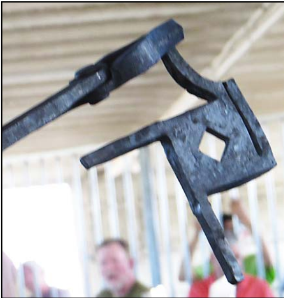
After bending out each leg, the tiny corner that remained was cut off. He left enough material there to refine the corner.
