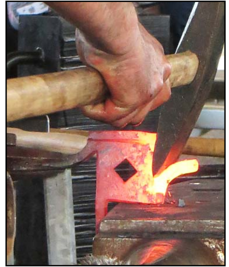
Slit with a hot cut along the strike lines.
