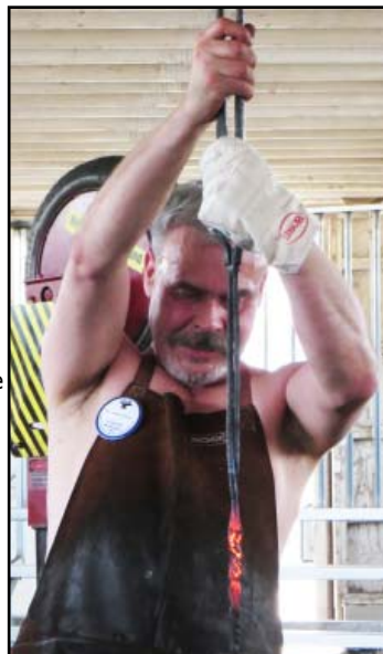
Forge weld loose ends. Gábor uses Borax, tossed on the piece while it is in the coals. Twist the doubled rod in the same direction as each leg was twisted, keeping twist even. Reheat and adjust as needed.
