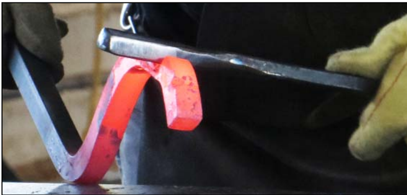
Flatten the bend at a high heat and with tenon form tool in place. Tenon pattern tools are made in swage for uniformity and consistency. This tool has an end profile of a dovetail but tapered.
