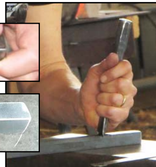
Left, drawing of the layout. Above center, photographs of the layout. Above right, scribing with a sharp chisel, and using the angle finder to mark 15°
