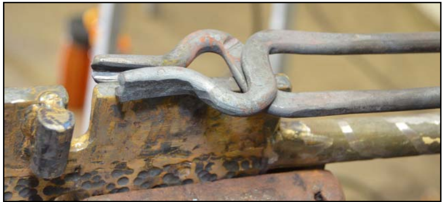
Tong jig and finished tong halves.
