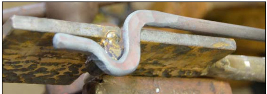
Finished tong half shown with jig.
