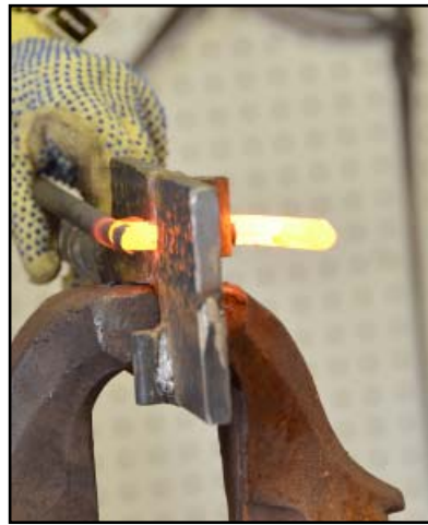
Tong jig in use.
