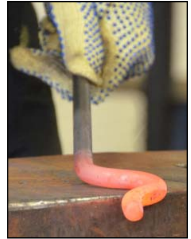
Round bar formed by jig.
