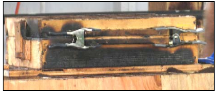
A mold for a core that would be used to create the eye in the hammer head. Matt said if he found a workable sand to make cores, he would have poured it with the core. .
