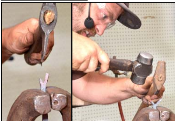
Opener jaws cut mark cleaned and radiused with fuller.
