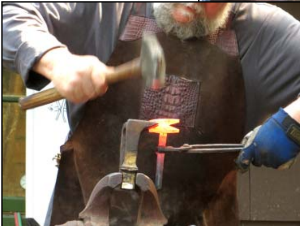
Bridge shaped anvil tool (placed in the vise because the demo anvil was not stable enough).
