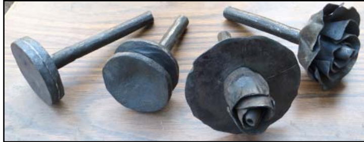
Starting material for this one piece rose was a 2 inch cube. Previously, Fred had forged the starting cube into a disk with a tenon on it, the far left piece as pictured in the photo above. The steps for forging the disk with tenon is seen in the diagram at right.
