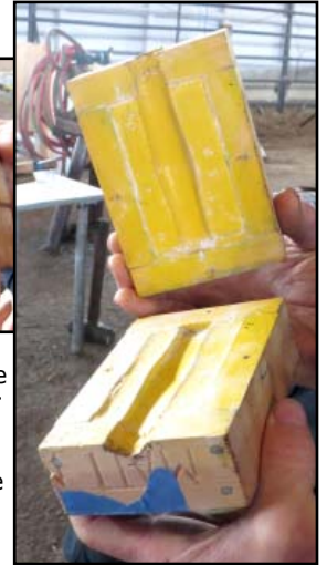
A mold for a core that would be used to create the eye in the hammer head. Matt said if he found a workable sand to make cores, he would have poured it with the core. .
