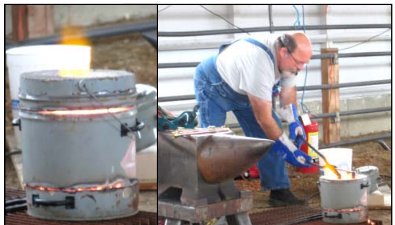
Crucibles are made of silicone carbide or graphite. Only one type of metal should be used in each crucible.
