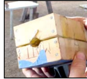
A mold for a core that would be used to create the eye in the hammer head. Matt said if he found a workable sand to make cores, he would have poured it with the core. .
