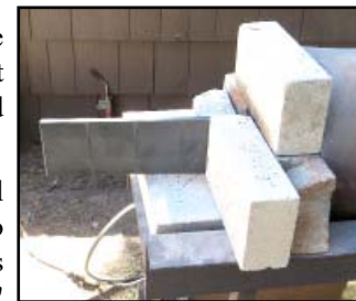
A fine example of hot cut sculpture. These two design element samples are each forged from one piece of steel (same design but the one on the left has more completed detail)
