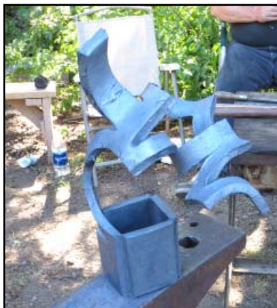
Fred bending the piece at the heat using a large bending fork.
