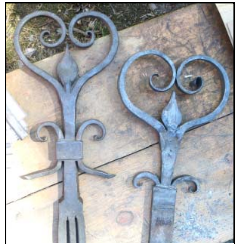
A fine example of hot cut sculpture. These two design element samples are each forged from one piece of steel (same design but the one on the left has more completed detail)
