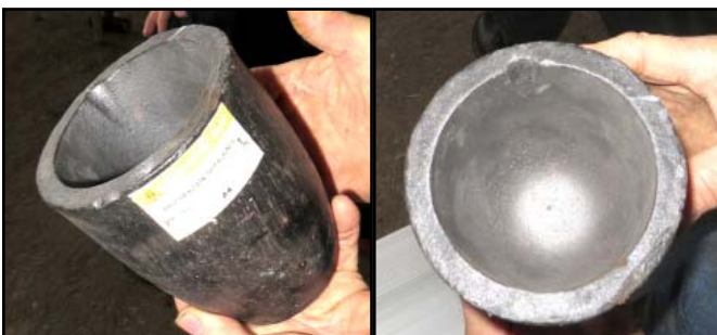
Crucibles are made of silicone carbide or graphite. Only one type of metal should be used in each crucible.
