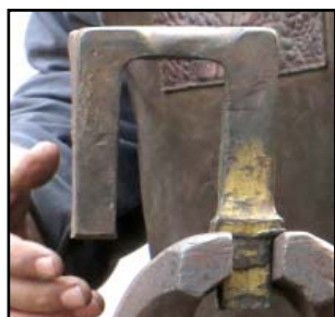
Bridge shaped anvil tool (placed in the vise because the demo anvil was not stable enough).
