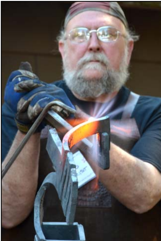
Fred bending the piece at the heat using a large bending fork.
