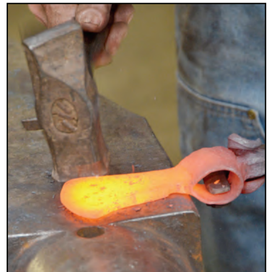
Note the tongs grabbing the eye while working on the blade in the final clean up.
